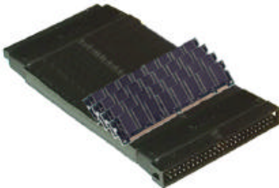
Figure 2b. Pass-through ATA connector implementation
